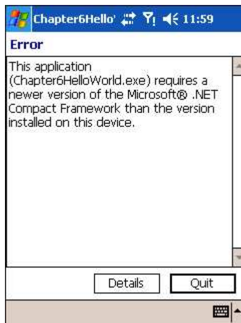
Figure 6-5. Error message displayed when attempting to run a .NET Compact Framework 2.0 application on a device without the version 2.0 runtime
