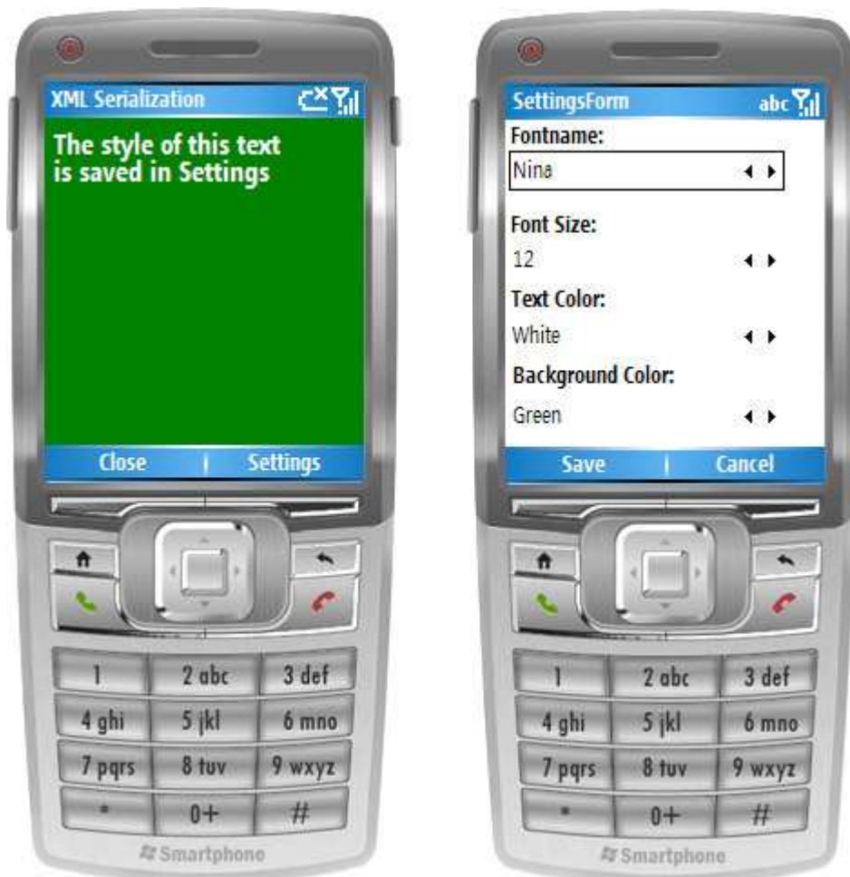
Figure 3-19. Screen of test application that stores graphics settings in a file stored using XML serialization
