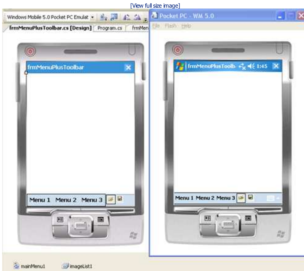
Figure 2-8. MainMenu and ToolBar controls, at design time (left) and at run time (right)
