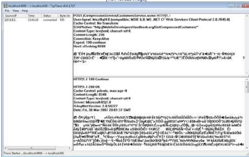
Figure 7-6. TcpTrace of the HTTP messages sent with the SOAP message compressed
