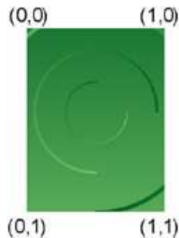
Figure 13-5. Texel coordinates in a texture
