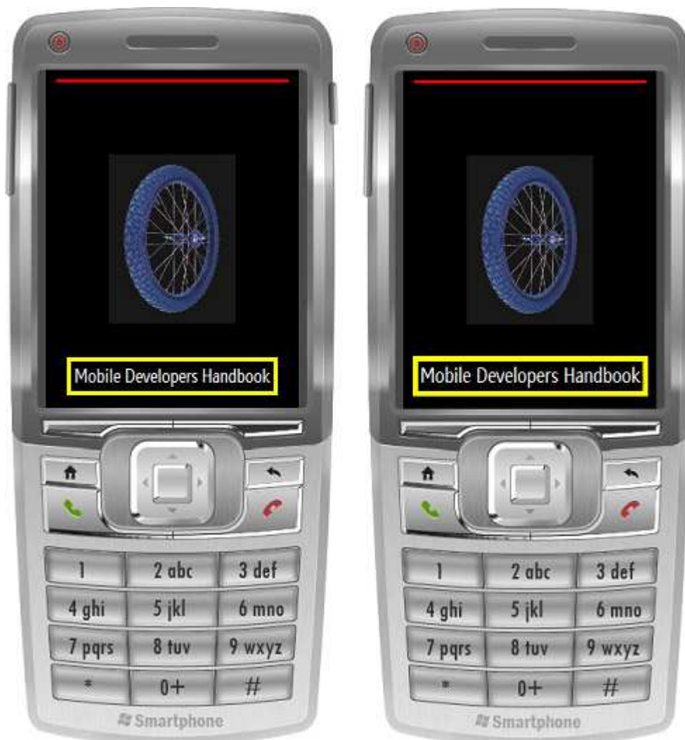
Figure 12-4. Increasing the pen width and font size on a high-dpi display (right) to counteract the shrinking effect
